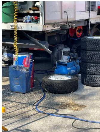
Spill trays under fuel drum and generator are not in place
