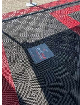
These types of mats need to have a second layer underneath to catch fluids running through the holes
